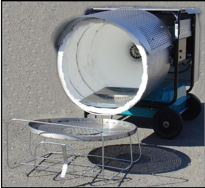
**Figure 15** – Combustion Chamber Cleanout Door
