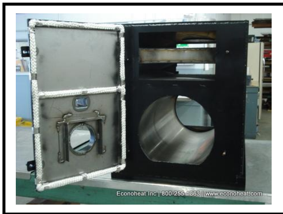
Figure 8 – Burner Door View
