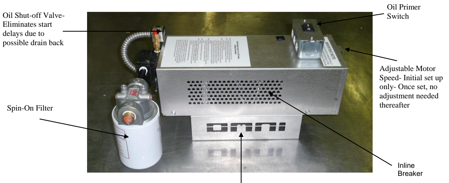
Figure 5 –Oil Pump Assembly
