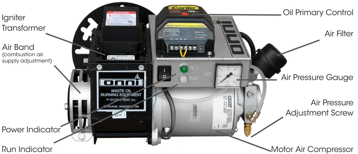
**Figure 1** - Oil Burner (Back View Closed)
